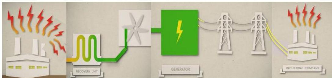
Waste heat stream is captured in the heat exchanger.
